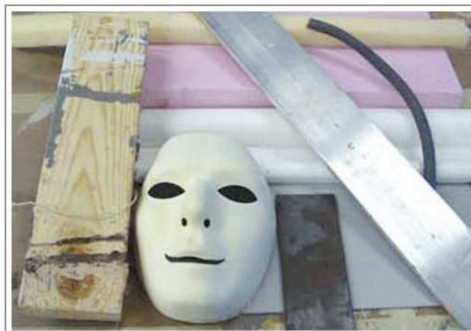
CrystalGel will adhere to a number of materials used in stagecraft. Some examples, show here, are upholstery foam, polystyrene, pine, aluminum, ethafoam road and steel.
