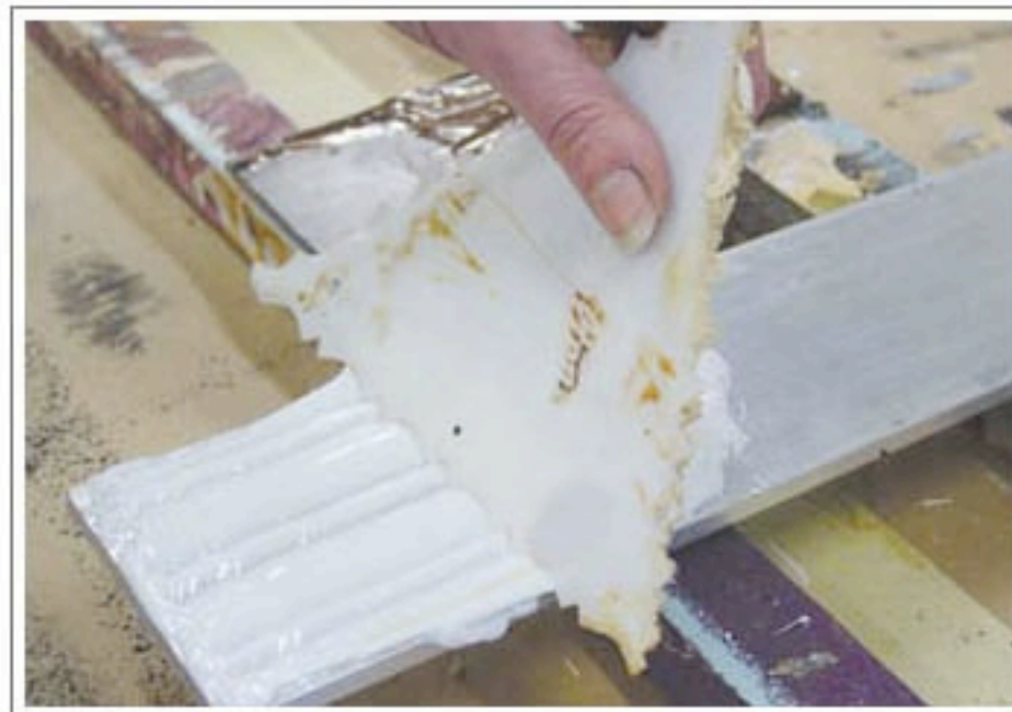
Many scenic artists will use a cake decorating tool for applying CrystalGel. It's shown here being applied to aluminum.
