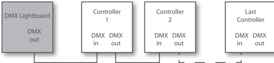
In configurations with use of a DMX lightboard the first controller can either be set in DMX mode 24 or in DMX mode 10 SYNC.<sup>2</sup>
