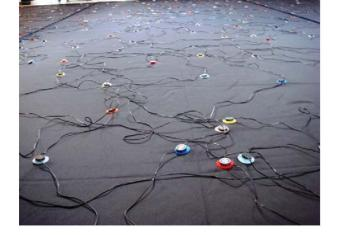
When you've placed the LED strings you it's necessary to measure out the cables so there's not too much cabling inside the starcloth. You can stick the end of the LED cable to the Floor with tape, then the cable continues to the place where the XLR cable will be attached to the strings.
