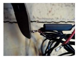
Slide the shrinking tube over all cables and use the lighter to shrink it.
