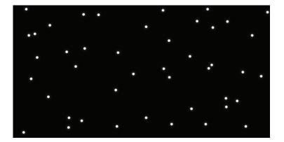
**Classic :** Spread the adhesive loop washers unevenly with clusters over the panel to get an irregular distribution of LEDs. Always put sockets from different channels in clusters.
