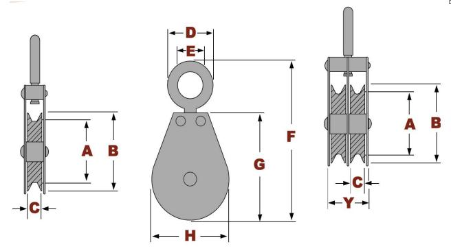
\*WLL=Working Load Limit [Based on a minimum 3:1 Design Factor]
