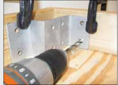
Using the LEG-A-MATIC™ as a template, drill four holes using a 1 3/32" drill bit.
