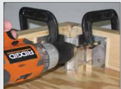
Using the LEG-A-MATIC II™ as a template, drill four holes using a 1 3/32" drill bit.
