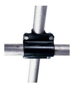
A fast and easy way to construct a pipe grid, these Gridlock Clamps are used at pipe intersections so that pipes can be installed wall-to-wall without cutting. Grade 5 bolts and locknuts are included. Works with Schedule 40 pipe.
