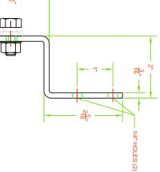
SHOWN WITH 1708 HANGING CLAMP, 1700 TRACK AND 1701 SINGLE CARRIER WHICH ARE NOT INCLUDED WITH THE 1722 WALL BRACKET
