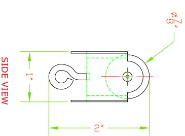
BODY MATERIAL - PLATED FORMED STEEL WHEELS - SOLID MOLDED NYLON RIVETS AND SWIVELS - NICKEL PLATED STEEL
