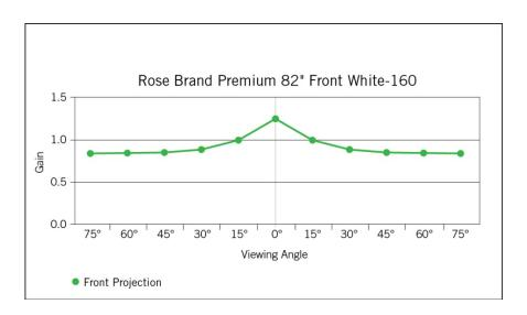
The standard for front projection where high gain is needed.
