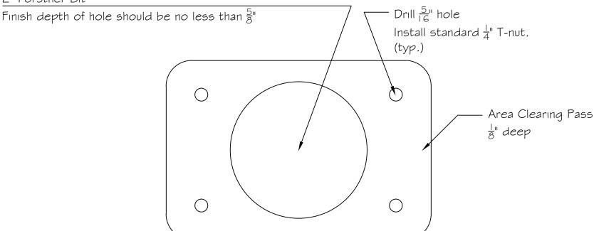
NOTE: Material is presumed  $\frac{3}{4}$ " thick. The depth of the hole drilled by the Forstner bit will remove all structural integrity in the remaining layers of material above the hole. It is presumed and recommended that there will be a surfacing layer (i.e. Masonite or MDF) to cover and distribute any weight in that area.
