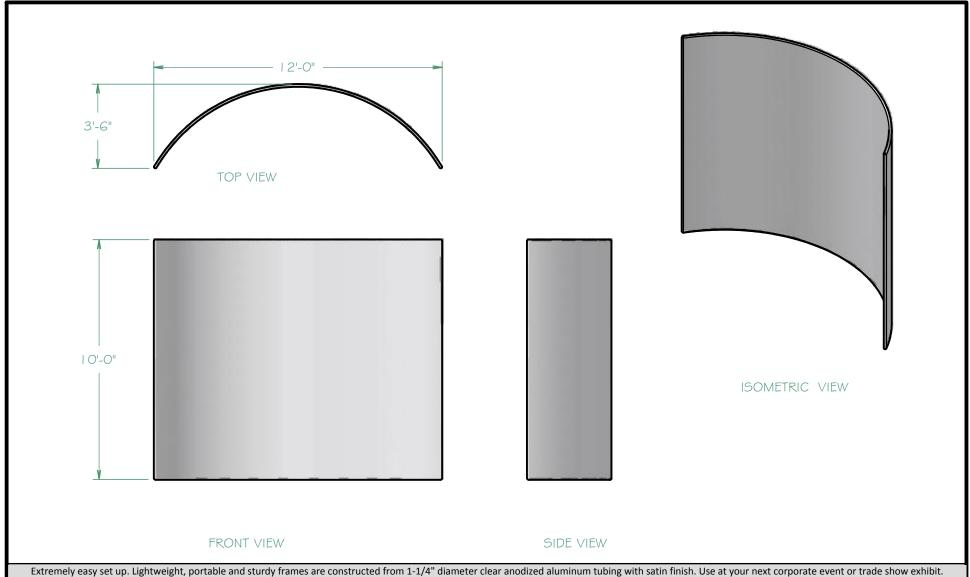
Extremely easy set up. Lightweight, portable and sturdy frames are constructed from 1-1/4" diameter clear anodized aluminum tubing with satin finish. Use at your next corporate event or trade show exhibit Travel Bag included.
