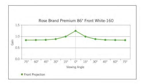
The standard for front projection where high gain is needed.
