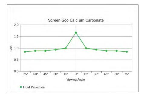
Projection has become a staple in performance, integrating seamlessly with scenic and lighting design. These standardized gain test results are a tool for helping to choose among Rose Brand's projection substrates. Many are materials specifically for high resolution projection, but also included are fabrics for more abstract lighting effects. As projection professionals know, gain/viewing angle is only one of many factors to consider when selecting a projection surface.
