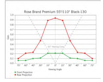
Great for show situations where the screen must not bounce ambient light. The screen formulation is ideal for using light in front of a video wall. It masks the individual pixels and results in a brilliant image with high contrast.
