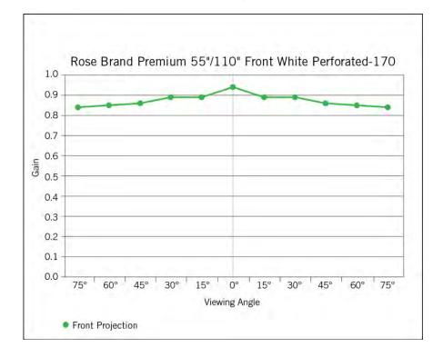
For acoustic transparency when placing speakers behind the screen.
