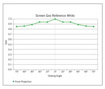
Best suited for rooms with complete light control - Use with projectors producing >12 ANSI Lumens per square foot of screen area. To create a Reference White Goo Screen you will need to apply **<u>both</u>** a Reference White Reflective Coat followed by a Reference White Finish Coat.
