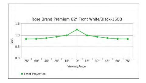
Front White material with an opaque black backing. The standard for front projection were high gain is needed.
